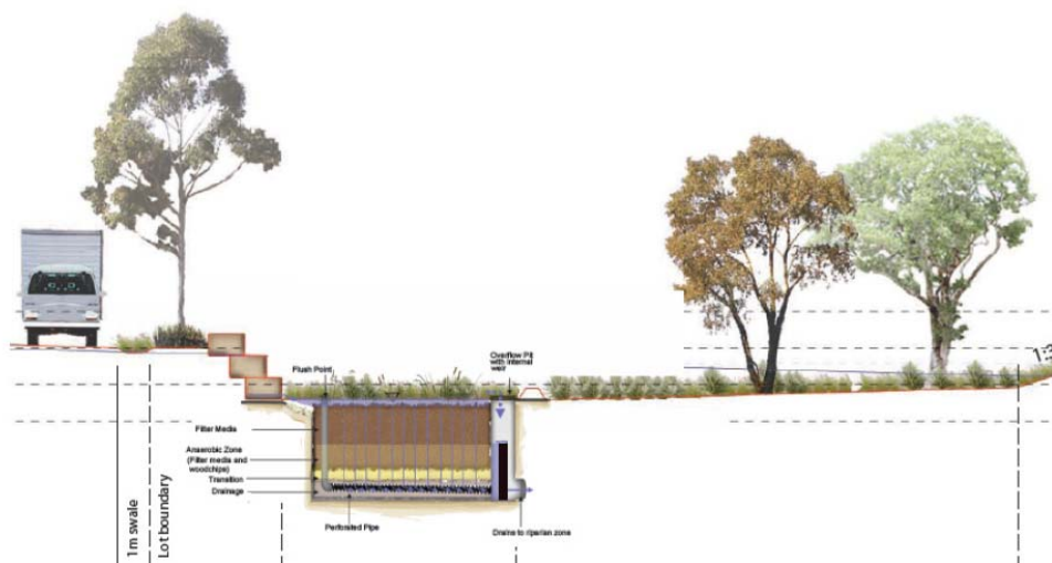
Figure 7.10 Section through detention basin showing a saturated zone bioretention and bund (small) separating it from the larger basin footprint
