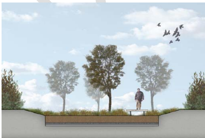
Figure 7.12 Section illustrating path within the detention basin
